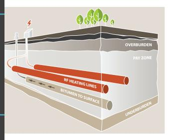
RF XL is a transformative RF heating technology that uses Silicon Carbide (SiC) generators, requires no dipole antennae, and has been proven in our 1/20 scale field test. In fact, Acceleware believes that we can now produce heavy oil and oil sands much more effectively and at much lower cost than SAGD.
